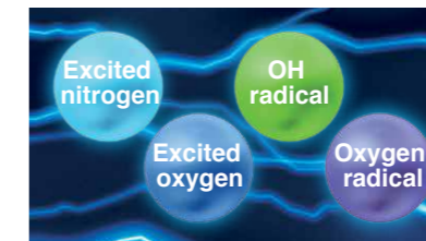
The electrons collide and combine with nitrogen and oxygen in the air to form four kinds of elements with powerful oxidative decomposition capabilities.
